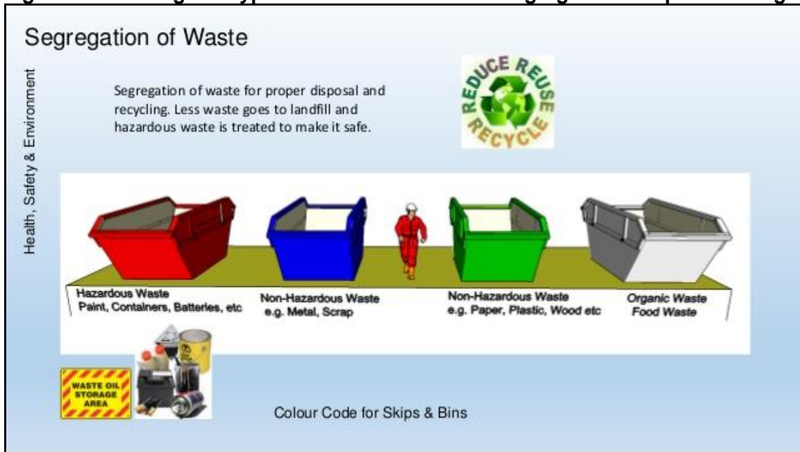
Figure 2 Image of Typical Construction Waste segregation compound design
